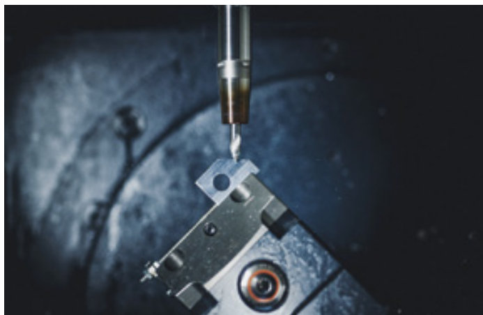
Milling cycle in the production of a joint piece using precise 5-axis CNC machining centres.
