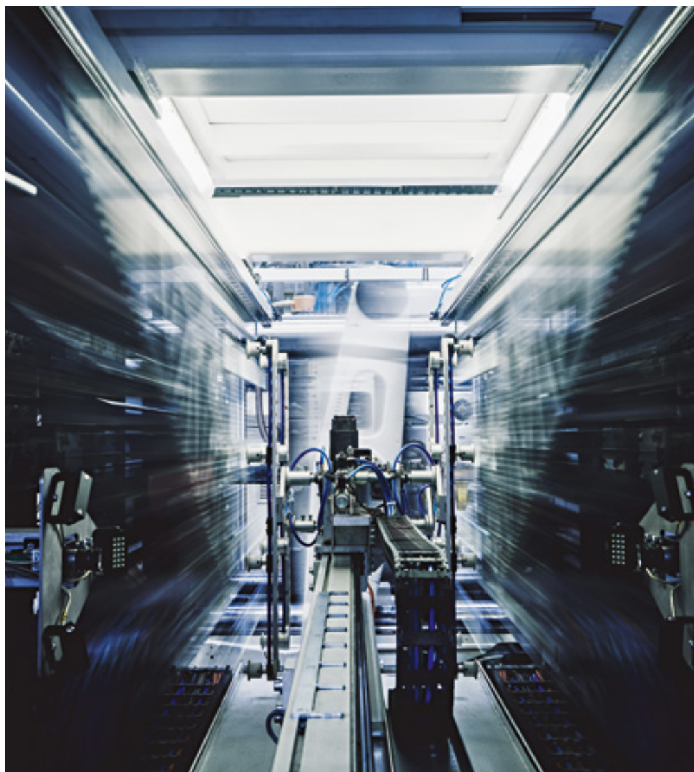
Production of cream cheese packaging High-speed transfer axis with video monitoring of an injection moulding production system
