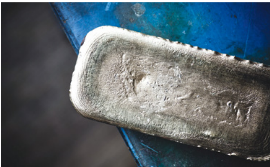
Small ingots made from melted scrap silver (e.g. necklaces, silver cutlery).
